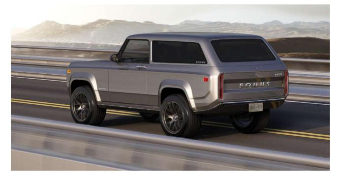
**EQUUS 4x4 e-concept** has an All-Wheel Drive management system thanks to four electric motor which develop up to 560 kW (750 + hp) and 820 lb.ft (1,100 Nm) of torque.
